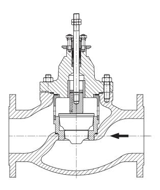
Valve with profile plug and pressuring cage
