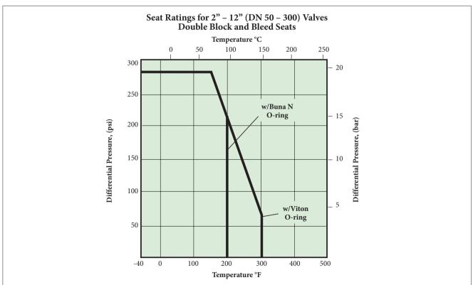
Valves are equipped with double block seats and the rating of the elastomer is the limiting factor insofar as temperature is concerned. Rating for standard elastomer Buna-N\* material is -40°F to +200°F (-40°C to +93°C). Rating for Viton\* elastomer is 0°F to 300°F (-17°C to +149°C). The standard DBB seat material is Filled PTFE.
