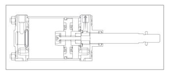
Perfect pneumatic cushioning produces minimal noise from end cover contact, and minimum piston deceleration time.
