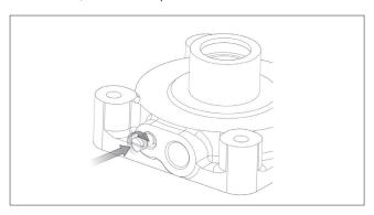
To achieve perfect cushioning, ensure cushioning screw is full open at the time of installation. Operate cylinder in full forward to full back. Now keep on tightening cushioning screw till cylinder stops knocking. This will give maximum life to your equipment and to pneumatic cylinder.
