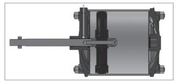
Perfect pneumatic cushioning produces minimal noise from end cover contact, and minimum piston deceleration time. To achieve perfect cushioning, ensure cushioning screw is full open at the time of installation. Operate cylinder in full forward to full back. Now keep on tightening cushioning screw till cylinder stops knocking. This will give maximum life to your equipment and to pneumatic cylinder.
