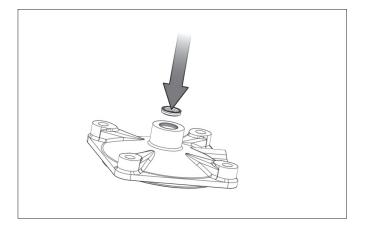
3. Place Cushioning seal (15) and o-ring (17) on its groove. Place o-ring (19) on cushioning screw (12), assemble the cushioning screw on rear cover (2).
