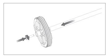
4. Insert this piston rod assembly carefully into the tube (3).
