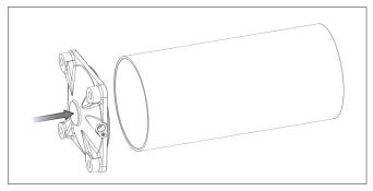
4. Assembled the cylinder cover nut (9) and tie rod (6) on rear cover (3) with tube (3).
