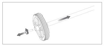
2. Remove lip seal (16) and buffer cap (10) from piston (4). Use blunt needle to remove lip seal (16).
