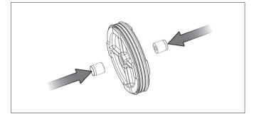
Apply drop of 7649 primer (dryer) on internal threads of piston rod. Wait for a minute and again apply a drop of 242 loctite on same threads. Now tighten the piston rod (5) with the help of SHC screw (8) by using washer (13).
