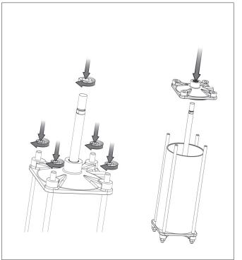
**NOTE:** Operate the cylinder assembly by hand. It should be free rotating piston rod & operating in and out.
