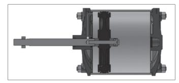
If cushioning is not provided then air passes through exhaust port only. When stroke comes to an end, piston strikes the end cover with some acceleration, giving rise to knocking noise, stresses on cylinder components and vibration transmitted to the machine structure.
