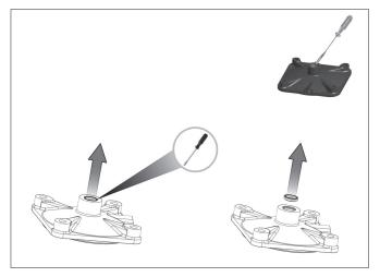
3. Remove o-ring (17) and cushion seal (15), take out cushioning screw (12) wiith o-ring (19) from front cover (1).
