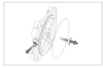
Clean tube (3) and rear cover (2) with liquid soap solution. After drying apply grease on rubber parts and inside the tube. Replace these rubber parts.
