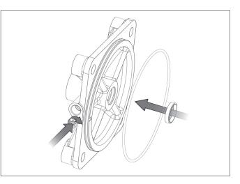
4. Assembled the front cover (1) on the tube (3), fasten the cylinder cover nut (9) and engage the lock nut (7).
