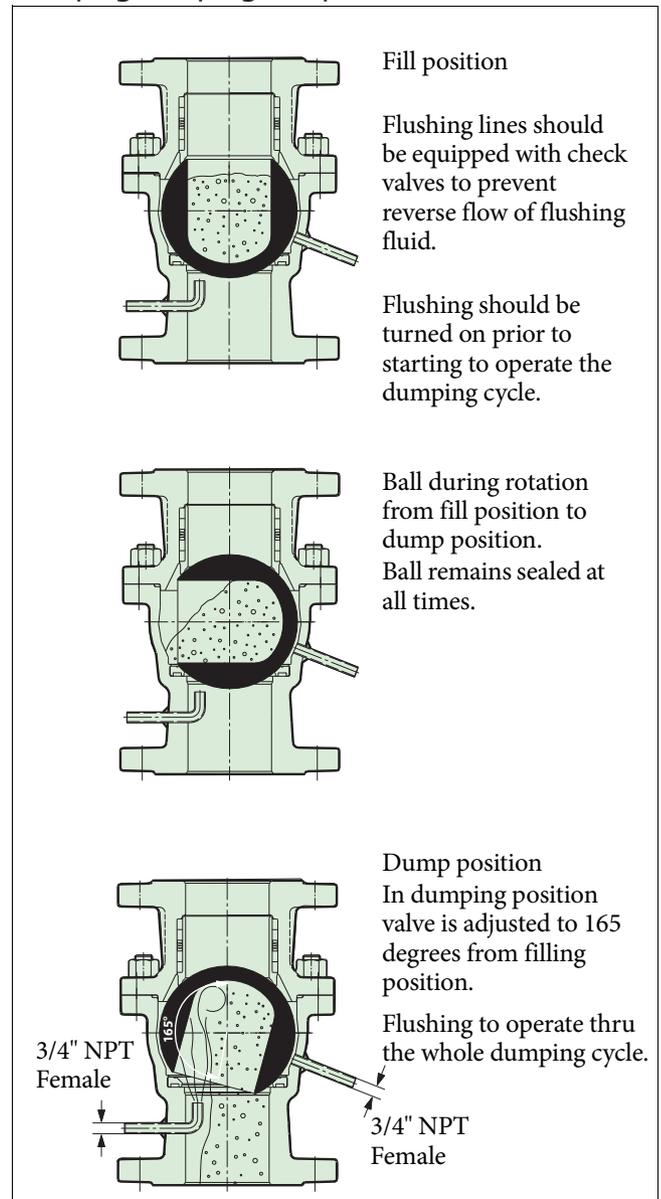
The figure shows the arrangement for filling the ball, starting the dump cycle, turning on the water purges and completing the dump cycle.
