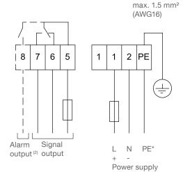
(2) With option Fail safe alarm (rotation control) Contact open when de-energised
