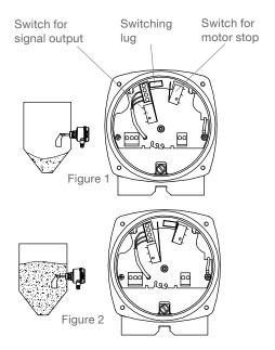
With the option fail safe alarm it is possible to recognize a fault of the unit in time and to initiate an alarm relay. The following faults are observed:
