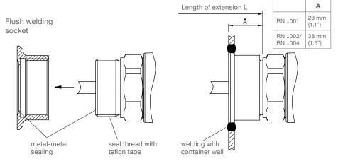
Dimension of flush welding socket (for optional on site manufacturing):
