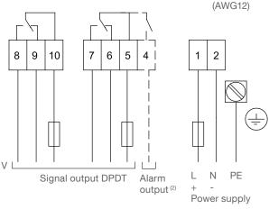
(2) With option Fail safe alarm (rotation control) Contact open when de-energised
