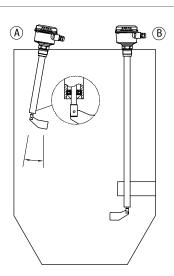
A Full detector vertical from the top max. "L"=3,000 mm (118")
