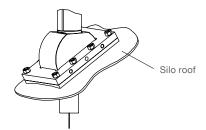
Flange plate outside dimensions: Width x Heigth: 120 mm x 180 mm (4.7" x 7.1")
